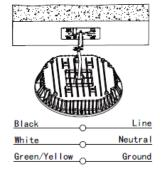
4. Slide fixture back into the connecting plate and replace the screw that was removed in step one
