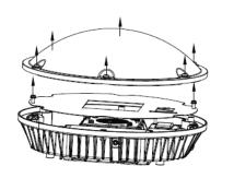
2. Reroute wires coming out of ¾" hole and seal the hole with provided plug. Drill 4 holes on four corners and fix it onto the ceiling with suitable screws.
