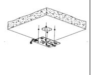
3. Buckle the connecting plate into the clips and connect the wires as shown below
