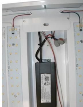
Channel cover comes out by removing (2) ¼-turn fasteners to facilitate driver access.
