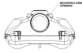
Determine the size of the mounting arm. This luminaire is designed to optimally accommodate a 2" mounting arm. If mounting to a 1-1/4" arm, use of included birdguard is recommended.
