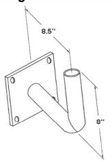
Application: For use with ELFL, LFL, or MEDF series Floods equipped with ELFLSF or MFLSF slipfitter bracket and when mounted to walls or other flat surfaces.
